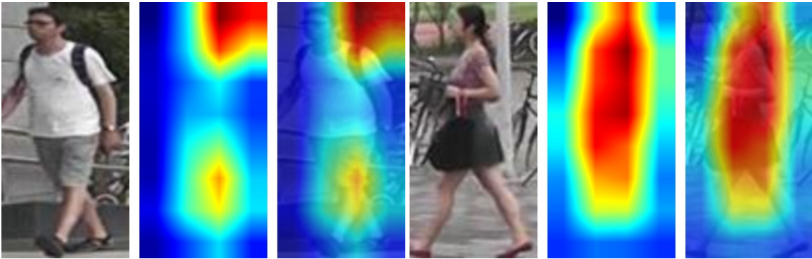
Figure 5.9: Activation maps from a model scrubbed for the person on the left (right set is not scrubbed). For each triplet, from (L to R) are the original image, the activation map and its image overlay. Note the effect of scrubbing: activations change significantly for the scrubbed sample (compare column 2 to 3) whereas remain stable for the non-scrubbed sample (compare column 5 to 6).
